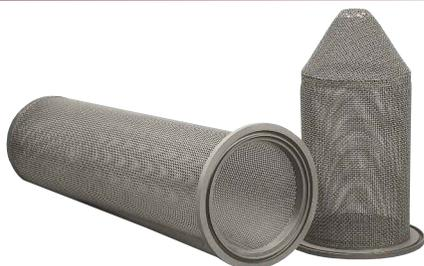
Perforated or Mesh Support Baskets and Specialty Baskets for AM/RB Series #1 and 2 size filter vessels are constructed of T-316 stainless steel. Specialty Baskets include Strainers, Mesh and Micron Lined Baskets, Canister Baskets, and Cartridge Chambers. These baskets require two O-Rings that fit into machined grooves on the top and the bottom of the basket flange.
