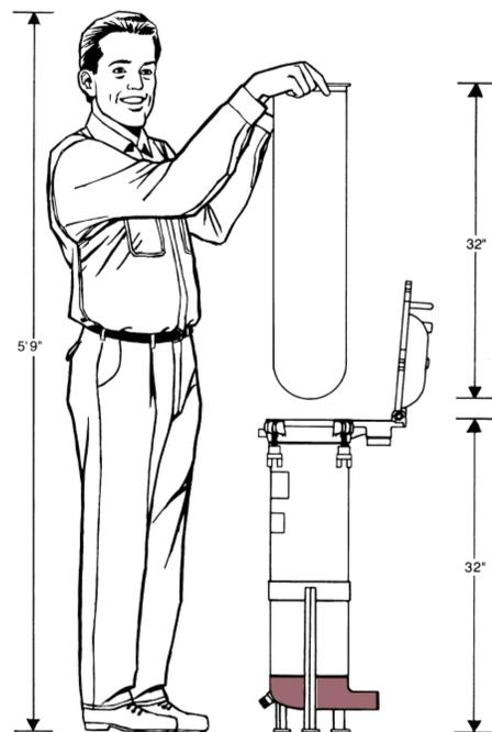
Lower working height means easier filter bag change-out for operators.
