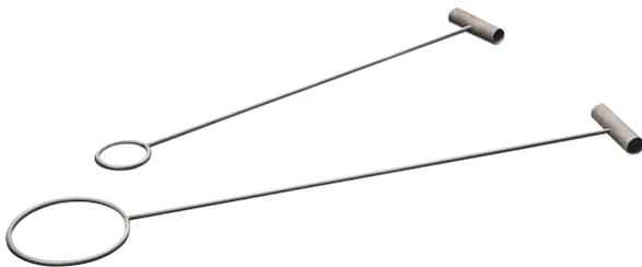
This accessory is designed to easily install filter bags, eliminating the need for technicians to reach into the bag during installation. The maximum surface area of the filter bag is used when the bag is properly seated and fully extended with this device. The Filter Bag Insert is fabricated of T-316 stainless steel and has a comfort handle.
