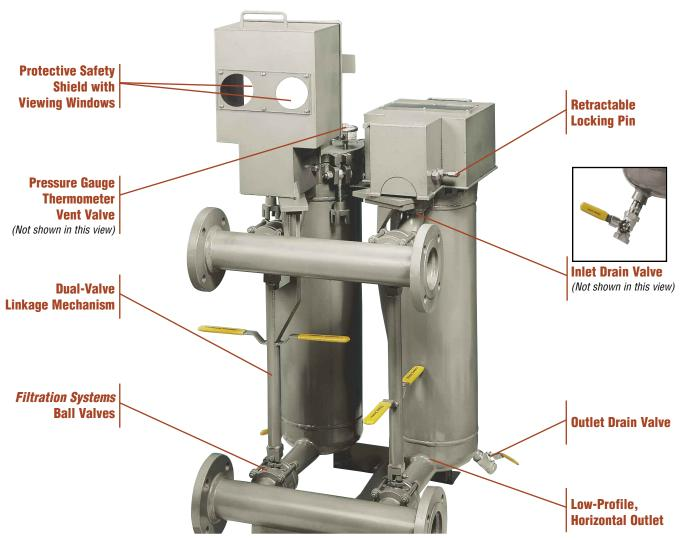
When in the closed position, the dual-valve linkage ensures that the vessel is "off-line" and safe to open. If either the vessel lid or Safety Shield is left open, the filter will not operate.
