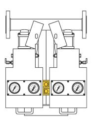
All **SAFEsystem**® vessels include a bracket for installation of a proximity switch (user furnished) to deactivate the pump. The use of a proximity switch can prevent a pump from being turned on accidentally.
