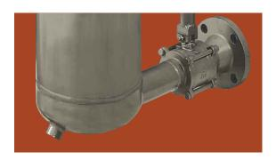
The low-profile outlet is a one-piece investment casting exclusive to the *Filtration Systems* product line and is an integral part of the *SAFEsystem®*. This design feature lowers the working height of our equipment, eliminating the need for a step stool or ladder when changing filter bags. Lower working height means easier filter bag change-out for operators. As a result, ergonomic-related injuries and accidental spills may be reduced.
