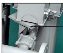
**Slotted Plate Locking Mechanism**
