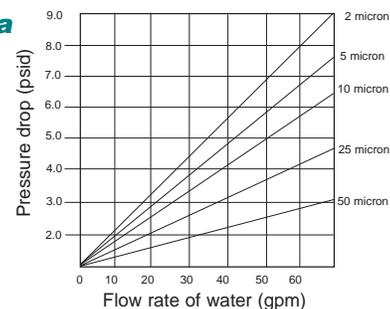
This graph does not include the pressure drop of a filter vessel, which should be included when sizing these products for your application.
