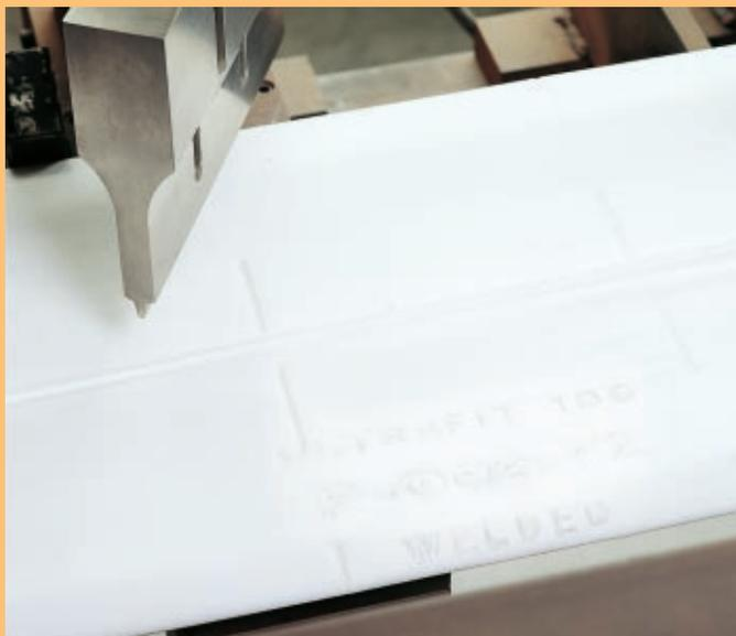
**Ultrafit** Welded Liquid Filter Bags have no sewn seams anywhere. Our patented ultrasonic welding process eliminates solids bypass.
