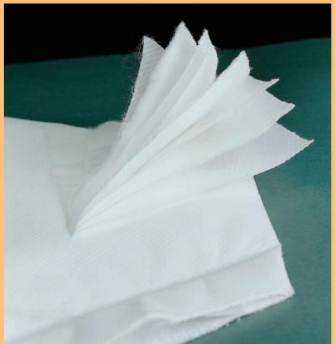
Constructed using a patented process of laminating multiple layers of non-woven material, polypropylene melt-blown microfibers are secured ultrasonically. Graded-density composite layers promote full-depth filtration and enhanced solids loading.
