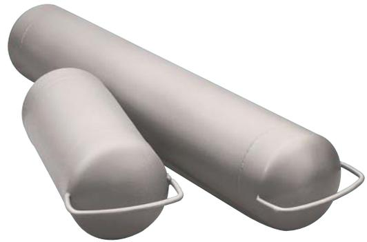
Placed into a filter bag prior to start-up, this accessory remains in the bag during the filtration process. When removed, liquid volume remaining in the bag is reduced, minimizing product loss and facilitating filter bag change-out. Liquid displacers are available in stainless and carbon steel for size #1 and 2 housings, and are equipped with a lift-out handle.
