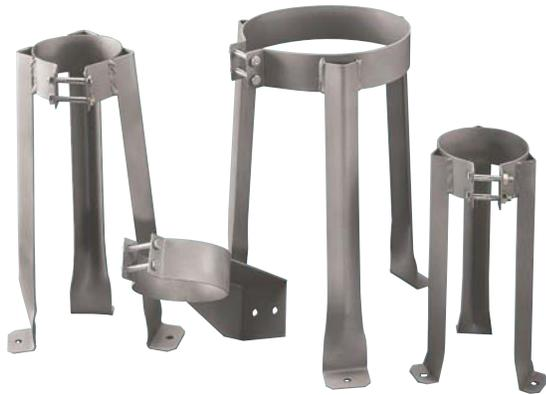
Available in stainless and carbon steel for size #1, 2, 4, and 5 filter vessels, these stands allow the user to raise and lower the filter vessel, as required. A Wall Bracket is available for mounting #4 & 5 size housings to a wall.
