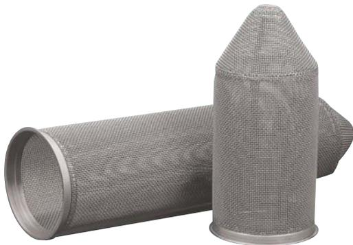
Type 316 stainless steel (8x8 mesh) basket accommodates filter bag sizes #1 and 2. These baskets have a tapered, cone-shaped bottom.
