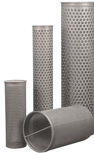
Heavy-duty perforated baskets convert size #1, 2, 4, and 5 filter vessels into high-capacity liquid strainers. When our filter housings are used with strainer baskets they allow heavy dirt loading at high flow rates. Perforated strainers are reusable and may be pressure cleaned, if required.
