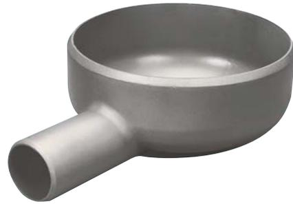
This one-piece, self-draining outlet, exclusive to the *Filtration Systems* product line, is optional on all #1 and 2 size filter vessels. This upgrade reduces filter bag removal clearance height by 4" on single vessels and 3" on modular systems, eliminating the need for a ladder or platform when changing filter bags. As a result, ergonomic related injuries and accidental spills during change-out may be reduced.
