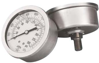
All *Filtration Systems* housings feature two gauge ports (1/4" NPT) to allow users to monitor both the upstream and downstream pressure. The variance between the two readings is called the *differential pressure*, and is used to determine when a filter bag is “blinding”, requiring change-out. Gauges have a 2-1/2" dial, 1/4" NPT connections, and are back-center mounted.
