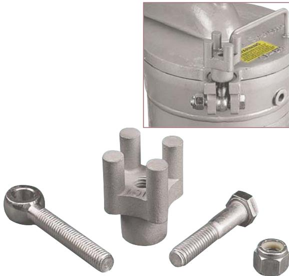
Replacement hardware is available in stainless or carbon steel for *Filtration Systems* ASME Code and Industrial Grade vessels. *Filtration Systems Over-The-Top™* vessels utilize four swing-bolt assemblies to secure the lid. A hardware assembly consists of four component parts: bar knob, eyebolt, axle bolt, and axle nut.
