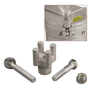
Replacement hardware is available in stainless or carbon steel for *Filtration Systems* ASME Code and Industrial Grade vessels. *Filtration Systems Over-The-Top*<sup>TM</sup> vessels utilize four swing-bolt assemblies to secure the lid. A hardware assembly consists of four component parts: bar knob, eyebolt, axle bolt, and axle nut.
