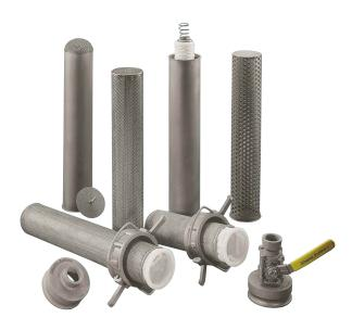
The Pipe-End Filter System provides effective, low-cost filtration without the nuisance or hazard of spillage. A shut-off valve isolates the filter during bag change-out, minimizing waste and employee exposure. Handles allow easy removal of the basket and filter bag. The quick-opening, cam & groove mechanism is easier to use than clamp-style, unsupported devices.
