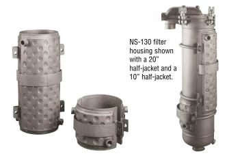
Thermal Jackets are used to maintain a desired liquid temperature during the filtration process. Jackets can accept steam, hot oil, water, heat transfer fluids, or refrigerants. The dimpled pattern design of our jacket provides highly efficient thermal transfer.
