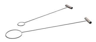
This accessory is designed to easily install filter bags, eliminating the need for technicians to reach into the bag during installation. The maximum surface area of the filter bag is used when the bag is properly seated and fully extended with this device. The Filter Bag Insert is fabricated of T-316 stainless steel and has a comfort handle.
